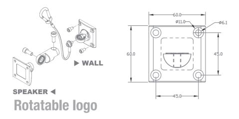
Depending on the mounting direction of the loudspeaker (either horzontally or vertically), the logo on the front grill of the loudspeaker that is held in place by a spring loaded mechanism can be rotated into the direction the speaker is mounted.
