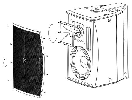
To rotate the VEXOlxxA's horn, the grille must be removed first. To do this, the eight screws on the sides must be unscrewed.
