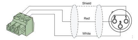
For unbalanced signal input connections
