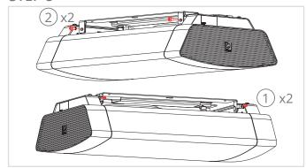
Keep the screw holes lined up and secure the screws in place. You can now release the NOBA8(A) and also secure the screws on the other side of the NOBA8(A).
