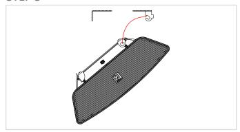
Hang the NOBA8(A) into the ceiling plate, making sure the mounting pins are fitted into the hooks on the ceiling plate
