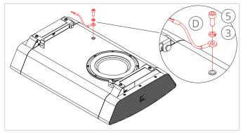
Attach the safety cable to the NOBA8(A) chassis
