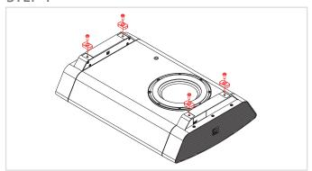
Remove the rubber feet by unscrewing the mounting screws
