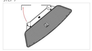
Rotate the other end of the NOBA8(A) up until the holes of the ceiling bracket line up with the holes on the NOBA8(A) bracket.
