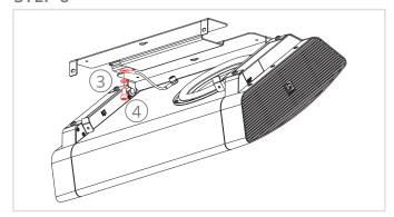
Mount the loose end of the safety wire to the safety bracket and make all electrical connections
