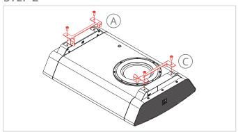
Attach the mounting brackets with the screws removed in step 1.
