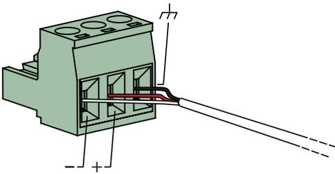
For unbalanced line input connections.
