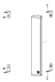
The L—shaped brackets have to be fixed to the wall through 2 screws. The used fasteners are depending on the mounting surface (brick, concrete, wood, ...) and should be chosen accordingly.
