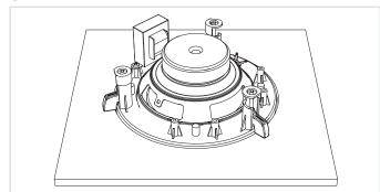
Fix the speaker in the provided opening by tightening the screws of the mounting clamps using a screw driver. A quarter turn will make the mounting clamps flip-out, locking the speaker in place. Tighten the screws for proper fixation of the speaker.
