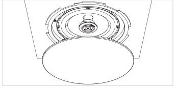
Attach the grill to the speaker by inserting the lips into the provided openings on the speaker baffle and rotating it over a partial turn (15°).
