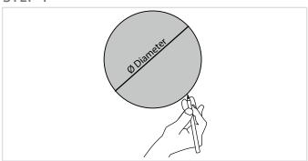
Cut a hole on the mounting location in the ceiling. Make sure the diameter is matching the cut-out measurement for the installing loudspeaker.
