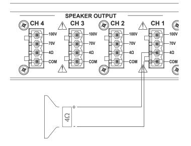
For operating using constant voltage (100V / 70V) audio distribution systems, all speakers shall be connected in parallel on the corresponding output terminals, non exceeding the maximum wattage / minimum impedance of the amplifier
