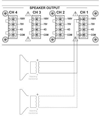
Depending on the chosen connection method (low impedance or constant voltage), the output configuration setup shall be configured accordingly.
