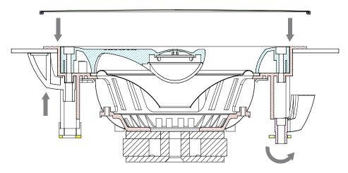
6) After the screws are tightened and the speaker is level with the surface, the front grill can be assembled to the loudspeaker.
