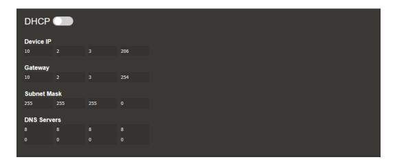
The DCHP function is standard switched off and can be turned one by clicking and enabling the corresponding indicator.
