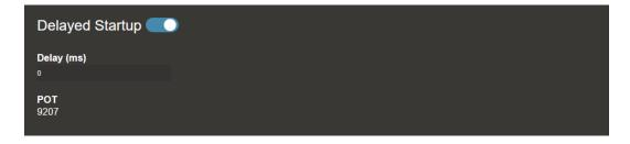
The delayed startup can be activated through enabling the indicated button, and the delay time (the delay between each two relays triggering) can be configured analogue (through a potentiometer located on the ARU20x PCB) or digitally through entering a milliseconds value inside the corresponding text field.
